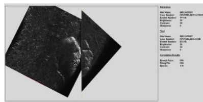
Photo 3: Ejector marks in two different weapons: Test fire & CS
